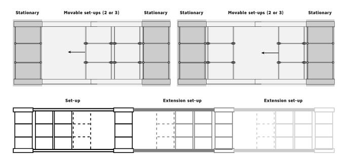
One UBeTrack<sup>™</sup> can consist of 2 or 3 mobile shelves. The total width can vary, see the illustration below. This can be increased in 25 mm increments up to a maximum of 250 mm which in turn alters the width of the walkway.
